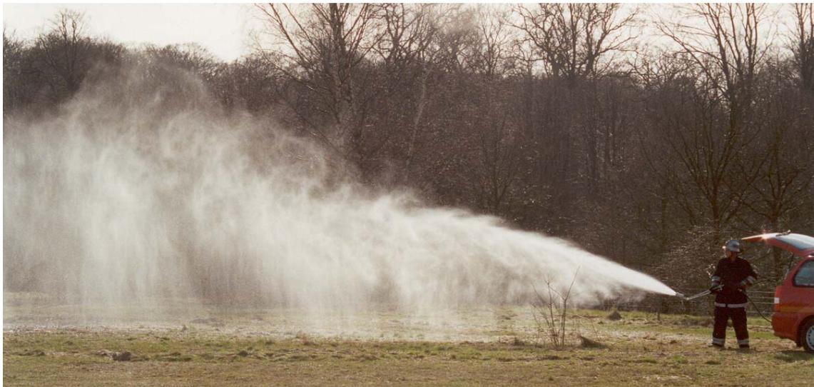
*The Firexpress HPU operates at a nozzle pressure (mouthpiece) as low as 23 bar giving the Micro-Drops a range of 15 meters.*
